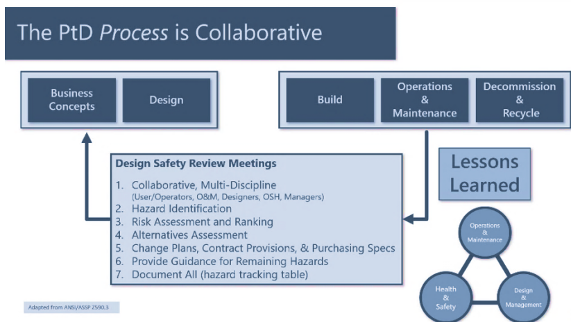
PtD collaboration process, adapted from the Z590.3 Standard (extracted from Jonathan Bach's Presentation)
